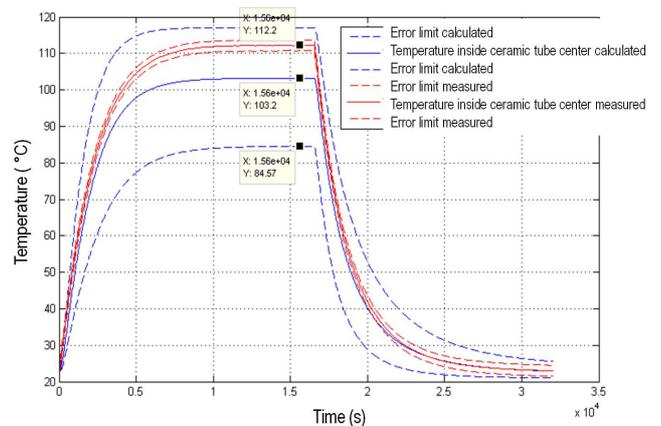
Fig. 11 Comparison of simulation and measurement of the temperature at metering point 4
