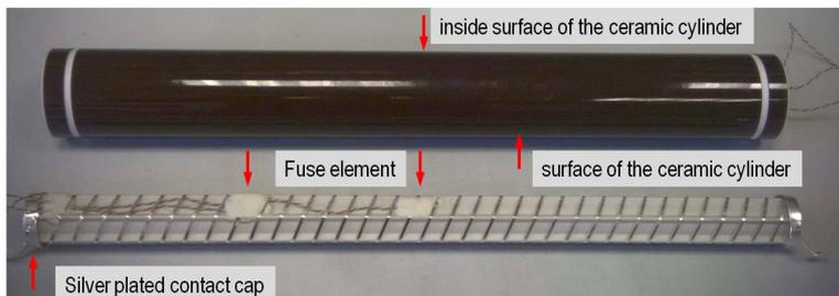
Fig. 9 HH fuse equipped with thermocouples inside and outside the electrotechnical porcelain, type SIBA HHD 40 A BU
