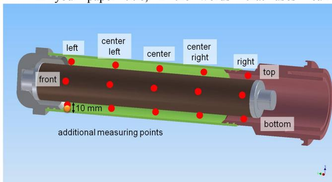
Fig. 3 Location of thermocouple inside switchgear and fuse tube accurately replace the word “using”, capitalize the “u”; if not, keep using lower-cased.
