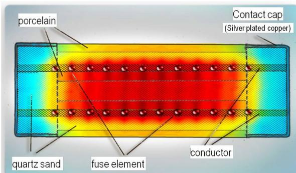
Fig. 7 Thermal model of the HH fuse in operation
