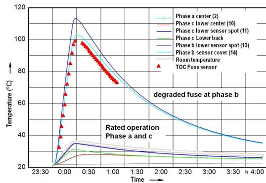
Fig. 6 Use of TOC fuse sensor and measured temperature distribution inside fuse tube while fuse with single broken fuse element is in operation
