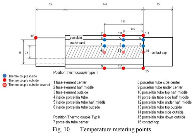
Fig. 10 Temperature metering points
