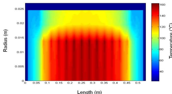
Fig. 8 Thermal simulation result at 35 A of the HH fuse type SIBA HHD 40 A BU
