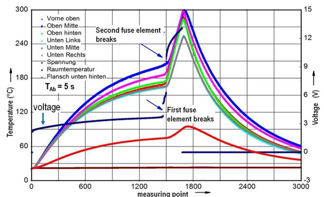
Fig. 4 Temperature distribution and time response while a first and second fuse element breaks
