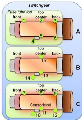
Fig. 5 Temperature measuring points inside fuse tube of gas insulated switchgear
