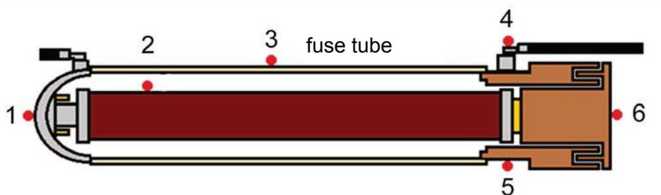
Fig. 2: Possible positions for thermal monitoring /5/
