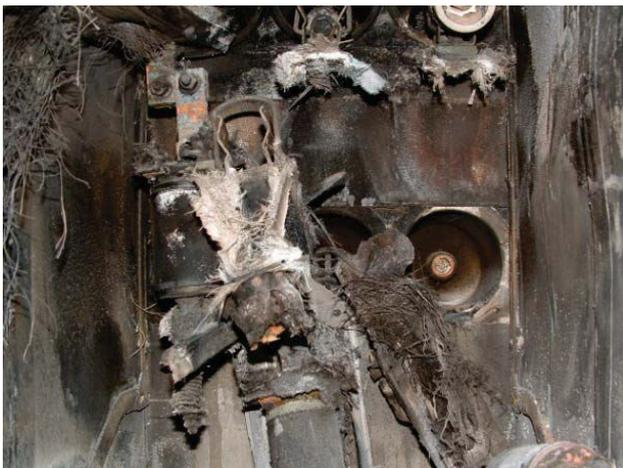
Fig. 1: destroyed medium voltage switchgear as a result of a blown-up HH-fuse
